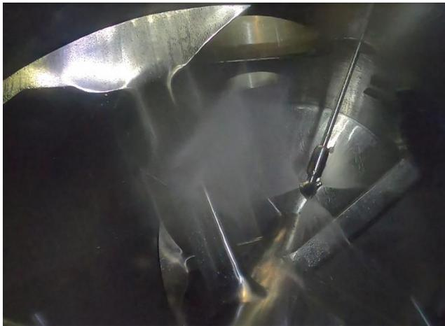
Rotating flat fan cleaning nozzle in a 10.000 l Lödige Ploughshare®-Mixer in operation. (Source: Lödige Process Technology)
