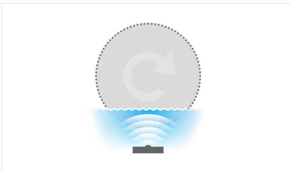
To speed up cleaning of the drum perforation, an ultrasound generator can be integrated in the cleaning system of the LC series*.
