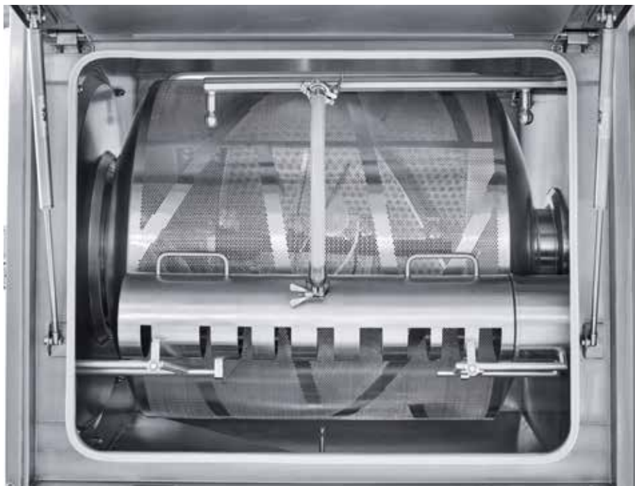
Inside view of a LC 70: the large inspection door enables good accessibility to the coater inside.
