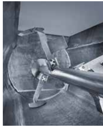
Ploughshare® Mixer type DBE with discharge door open: opening angle 90°
