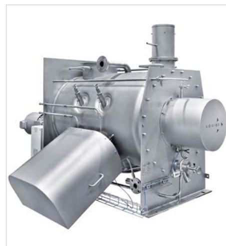
The covering above the bearing housing and motors creates an easy-to-clean surface
