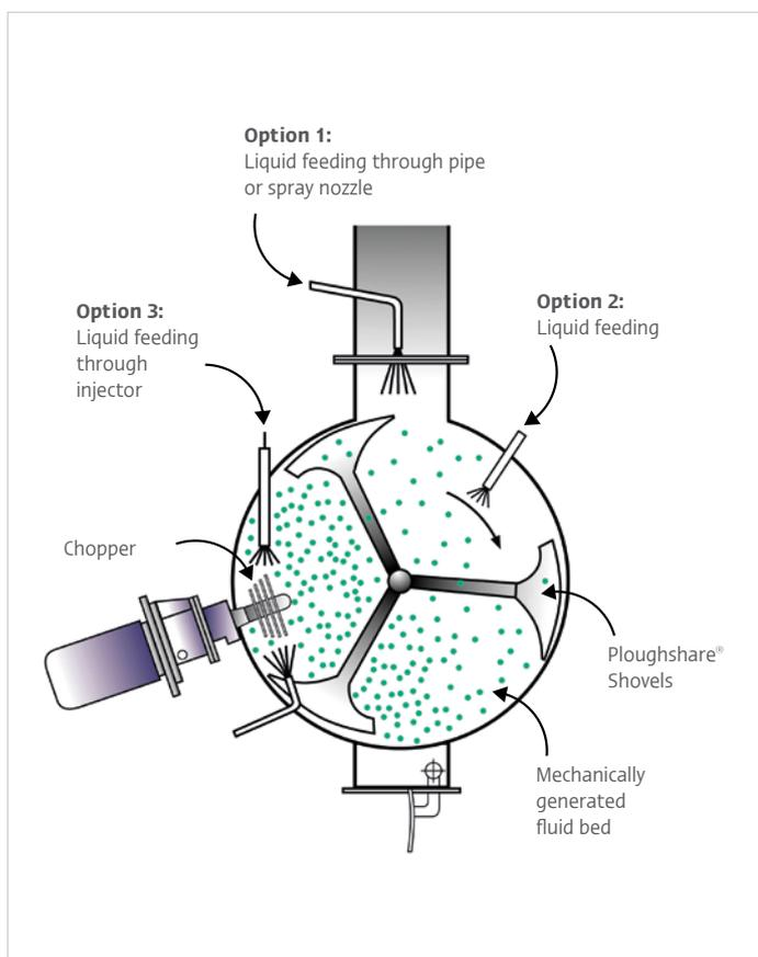
Some liquid addition possibilities in the LÖDIGE Ploughshare® Mixer following the principle of the mechanically generated fluid bed
