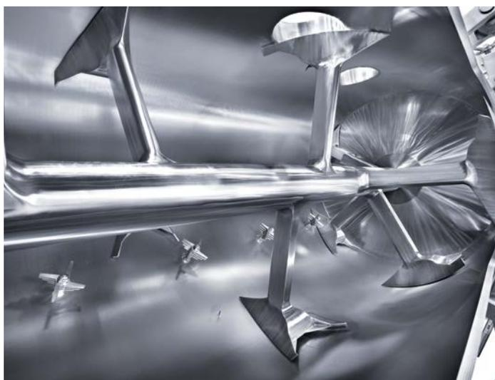
Welded mixing elements in hygienic design
