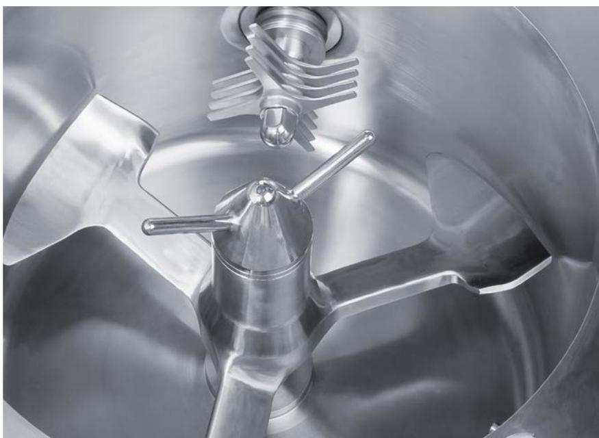
Mixing tool with tool lifting unit
