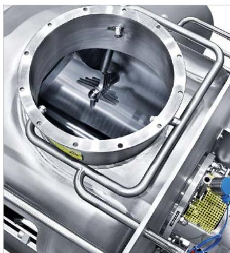
Cleaning nozzles for the WIP process
