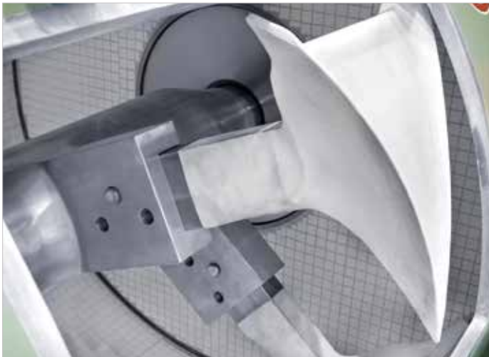
Ploughshare® Mixer for Li-NMC battery pastes
