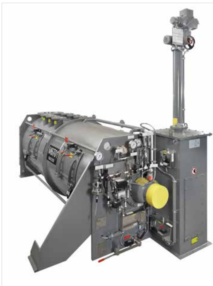
Ploughshare® mixer for continuous operation type KM in explosion-proof design for base stabilization of polyolefins
