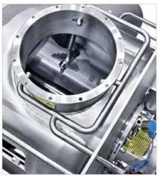
Cleaning nozzles for the WIP cleaning process
