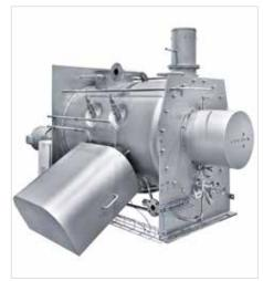
The cover hood above the bearing housing and motors creates an easy-to-clean surfaces
