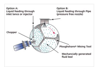
Some liquid addition possibilities in the Lödige Ploughshare  $^{\rm I\!B}$  Mixer following the mixing and fluidisation process
