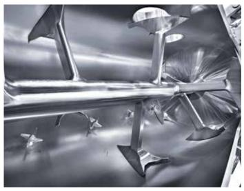
Welded mixing unit in hygienic design
