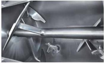
Fixed welded mixing unit in hygienic design
