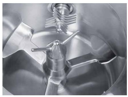
Mixing tool with tool lifting unit
