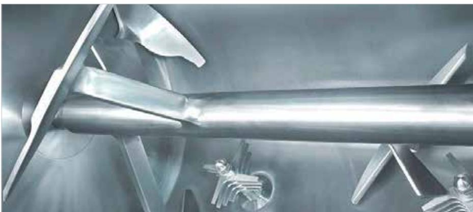
Fully welded mixing elements in hygienic design
