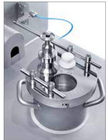
1 l vessel with PTFE inlet for feeding and thermometer
