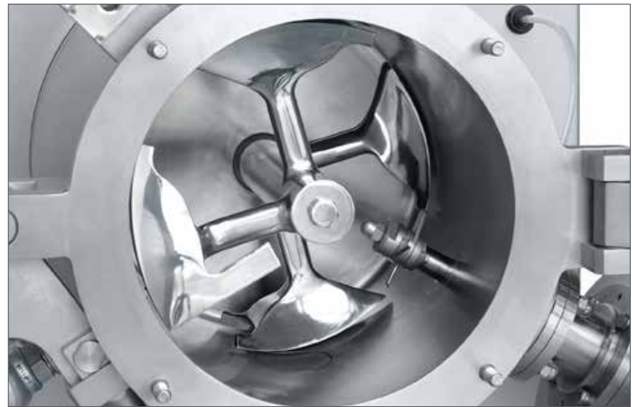
View into the mixing drum
