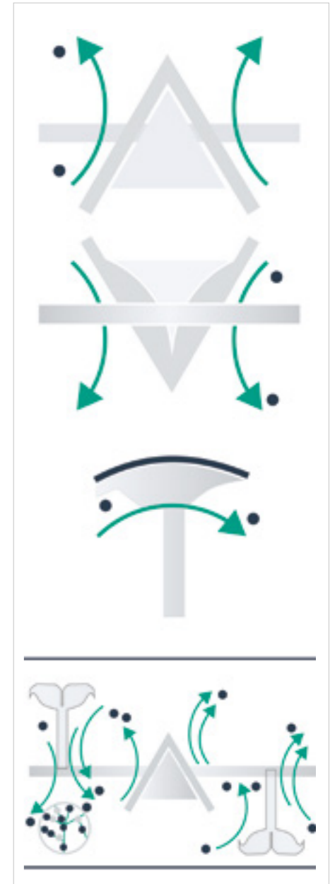
Principle of the mechanically generated fluidised bed.
