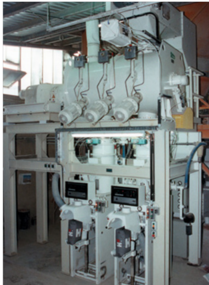
Lödige Ploughshare® Mixer type FKM 1200 D with automatic bagging
